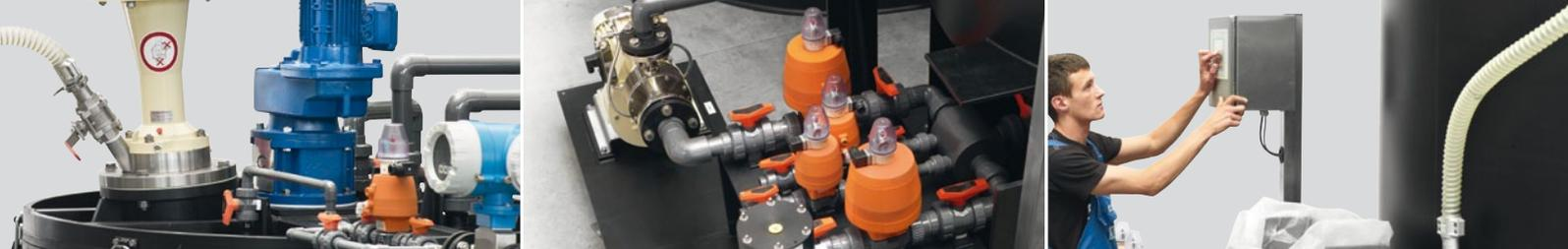
From left to right: Connection points for adding liquid, valves and high-performance disperser; separate heat exchanger for reducing temperature; monitoring the process states
